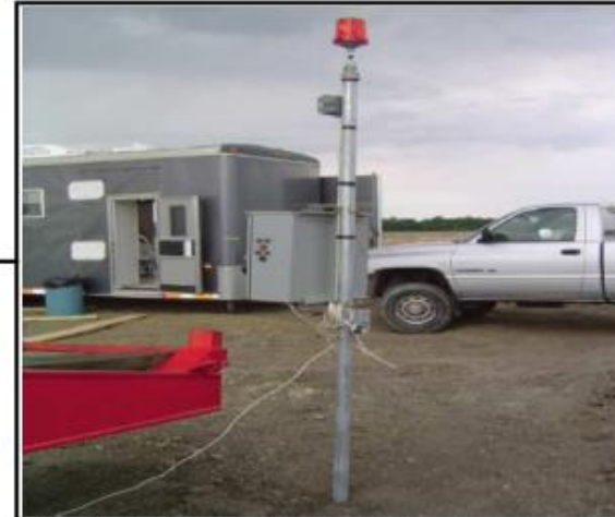
Figure 8 Ambient CO2 monitor with equipment trailer in the background
