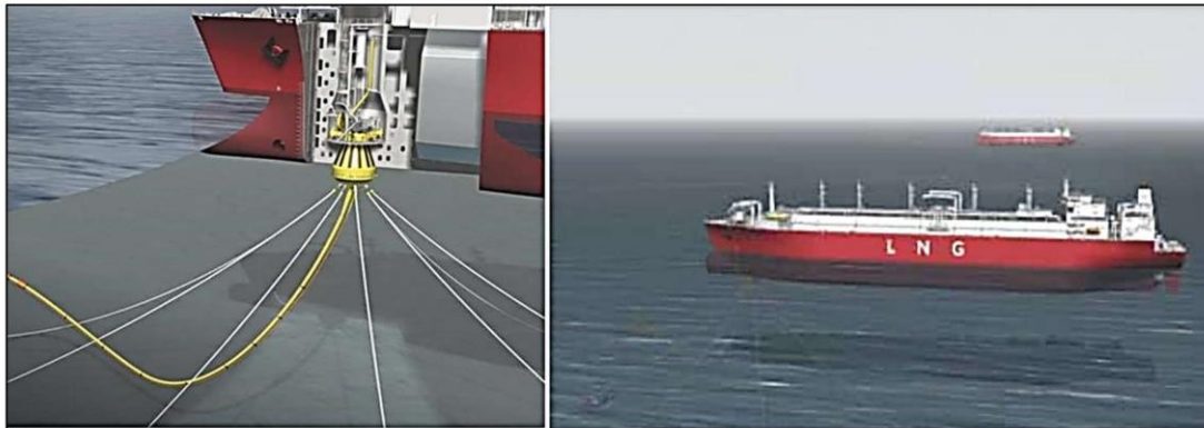
Figure 4-27 FSRU with mooring and loading system (source APL Offshore)
